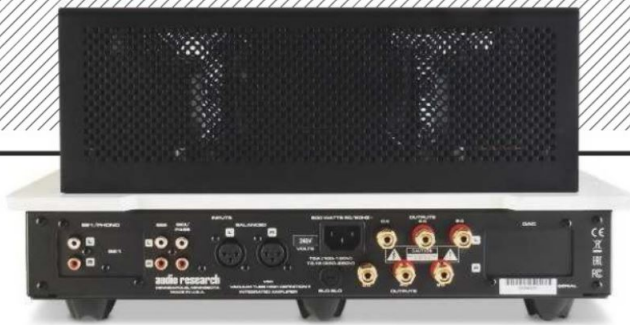
ABOVE: Three single-ended line ins on RCAs (one pass through) and a balanced set on XLRs are joined by 8 and 40hm speaker taps on gold-plated 4mm binding posts. Note spaces that will accommodate the phono [left] and DAC [right] modules
