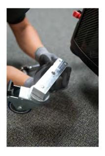
**17.** CAREFULLY THREAD THE M-POD INTO THE REAR OF THE M2 BASE AND LOWER THE M2 ON TO ALL 3 M-PODS
